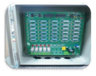
The Motor Controller is a Solid State Sequencer, specially designed for Rapping Motor Control in ESP System. The design enables to select any sequence for number of electrodes. Thus gives full flexibility to program the Rapping System at site as per the nature and amount of dust of that plant.
