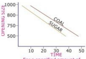
For a specified amount of material discharge through the different size of gate
